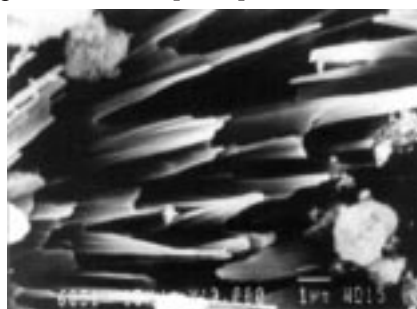
Fig. 2 Electron micrograph showing the needle-shaped morphology of the original sample No. 1, magnification 10 000×
